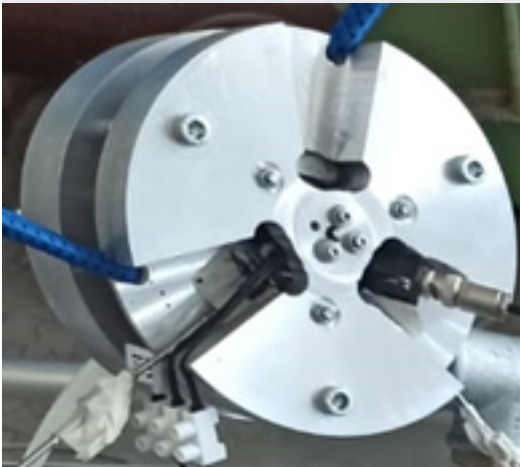
Tesla expander connected to an high speed generator
